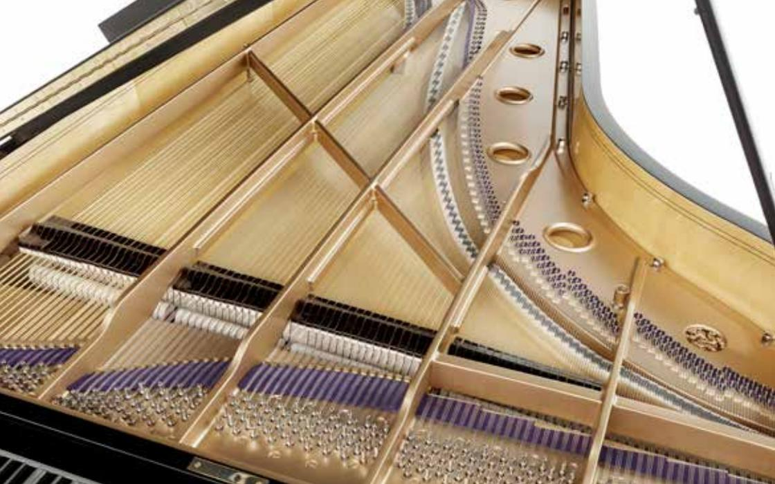
To hold the immense string tension (up to 20 tons), the cast-iron frame is an essential component since it has to give the necessary strength to the instrument.
