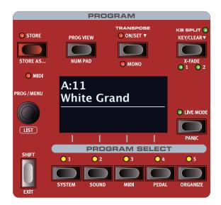
The Program section contains functions such as loading and storing programs, access to Live programs, keyboard split functionality and more. This is also where menus containing *System, Sound* and *MIDI* settings are found. The menus and their settings are covered in a separate chapter, starting on page 22.
