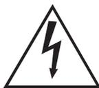
The lightning flash with arrowhead symbol, within the equilateral triangle, is intended to alert the user to the presence of uninsulated “dangerous voltage” within the product’s enclosure that may be of sufficient magnitude to constitute a risk of electrical shock.
